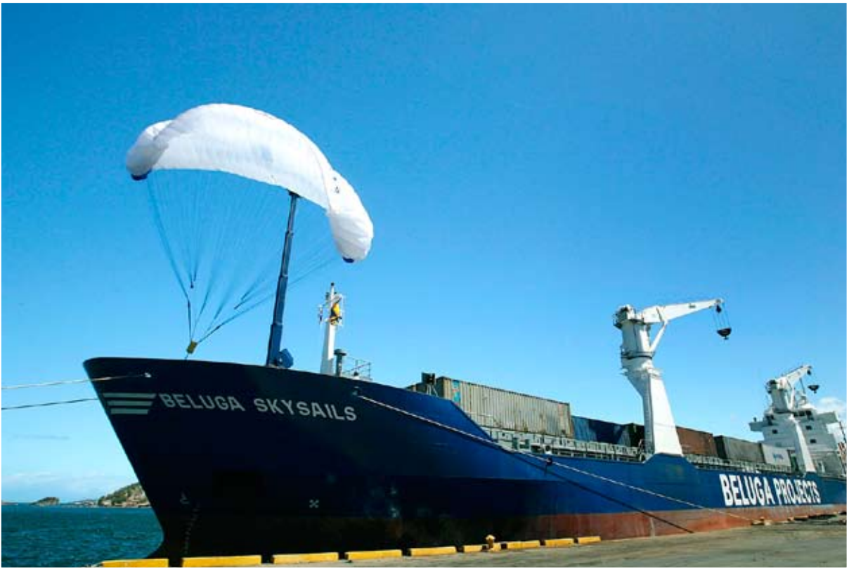
SkySails engineer Stefan Wartmann, above, stands under a kite onboard the MV Beluga SkySails in the port of Guanta in the city of Puerto La Cruz, 320km west of Caracas, in February 2008. The MV Beluga SkySails , a bulk carrier, was the first new-built ship equipped with SkySails kite system. Since 2008, the giant kite has helped the vessel reach ports across Latin America, Africa and Asia.
