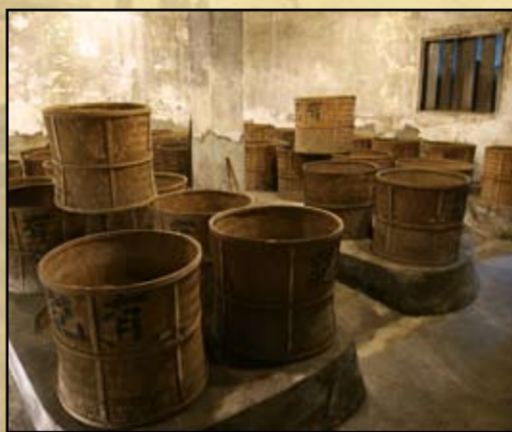
Tea leaves are roasted in bamboo baskets over charcoal fires in Youji Mingcha's curing room.
