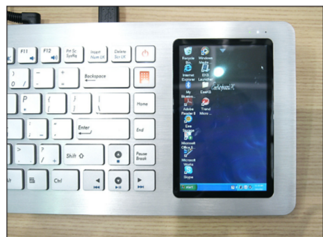
Asus' EeeKeyboard PC EK1542 is actually an all-in-one computer that runs Windows XP.
