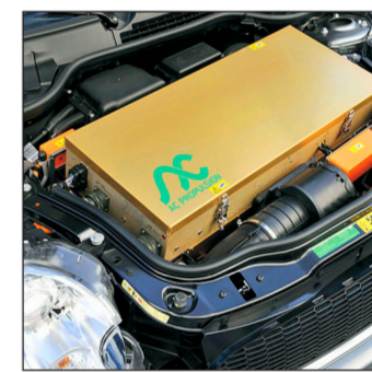
Above: Under the hood, a large box contains the electric motor, capable of pumping out around 200 horsepower.
